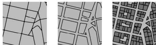
Figure 10: Left: Resulting street map. Middle: Blocks created by scaling from street crossings. Right: The generated lots. Allotments too small or without street access are removed.
